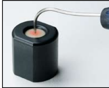
Light is red at the beginning of calibration step.
